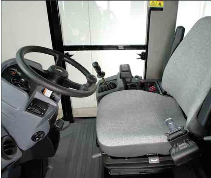
**Operational gauges.** Steering console and instrumentation gauges are infinitely adjustable within the tilt range to the desired position of the operator. Entire console tilts for simple entrance and exit.
