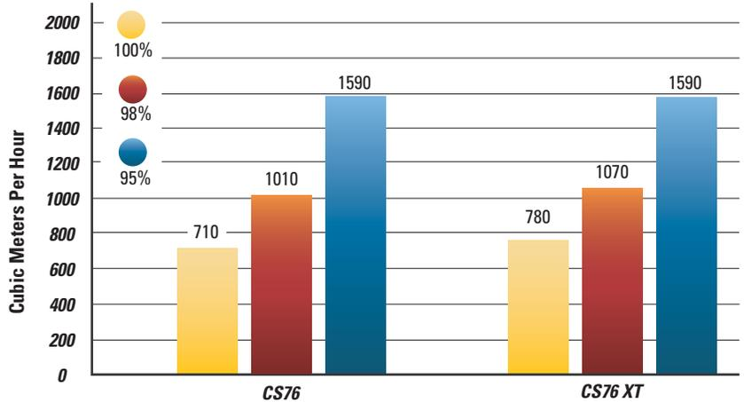
% Compaction of Standard Proctor
